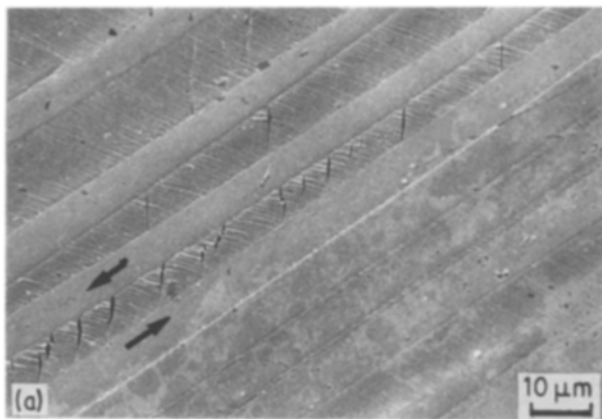
Figure 14 Higher magnifications of the damage zone ahead of a mode II crack in CF/PEEK: (a) 0.25 mm ahead; (b) 0.12 mm ahead; (c) 0.06 mm ahead.
